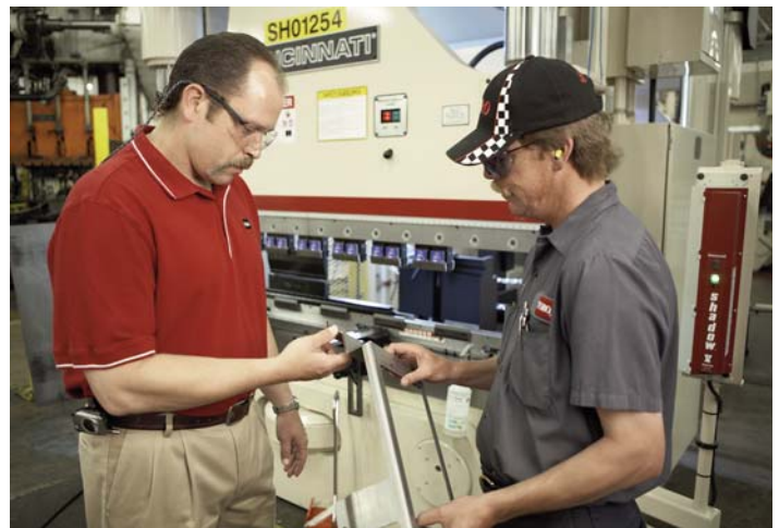
▲ Principal Manufacturing Engineer Rob McArdell, left, inspects a part. McArdell spearheaded an effort to modernize Toro's forming processes, which included upgrading to CNC press brakes and hardened, precision-ground, quick-change press brake tooling.
